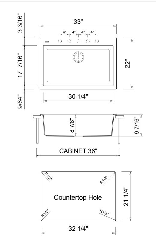
**NOTES:** Refer to installation instructions supplied with kitchen sink for undermount, or drop-in installations. Templates and installation kits provided with the sink.
